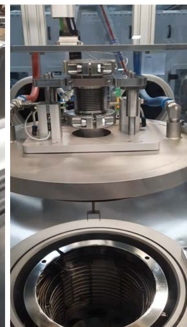
Dip furnace with automated controls – can run static corrosion experiments lasting 100s to 1000s of hours
