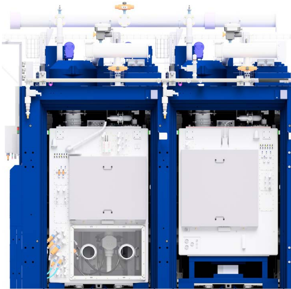
Cross-section view of new hot cells with integrated scientific instruments
